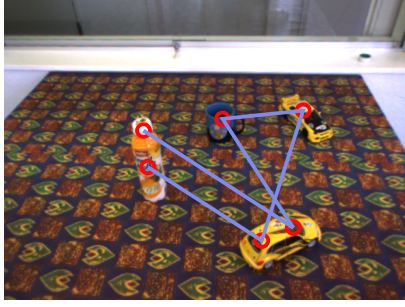
Fig. 7. The attention system generates a gaze pattern (blue) which is composed of a set of fixation points (red). The fixation points are used as seed points for object segmentation in the foveal images.
