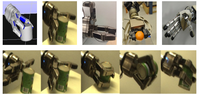
Fig. 4. (Top) Five robot hands used to collect databases described in Section IV-A. (1) Model of the 3-finger Schunk Dexterous Hand (SDH), (2) 3-finger SDH, (3) 3-finger SDH with Weiss tactile sensors, (4) 2-finger Schunk Parallel Gripper, (5) 5-finger iCub hand. (Bottom) Example of grasp execution with the SDH applied to the Can Cylinder (SD-5 database). Figures are reproduced with permission from [8], [23], [29].
