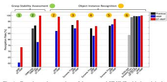
Fig. 4. Experimental comparison of the proposed ST-HMP with the original HMP, and the previously published results [1]–[3], [18]. The numbers above the images indicate one of the six database id. We evaluated our method for two tasks: grasp stability assessment (1-2 bar groups) and object instance recognition (3-7 bar groups). Support Vector Machines (SVMs) with a linear kernel were used as a classier in all cases. We closely followed the setups from the previous publications.
